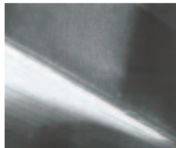
Wear of cutting edge (After cutting 1,800m)
